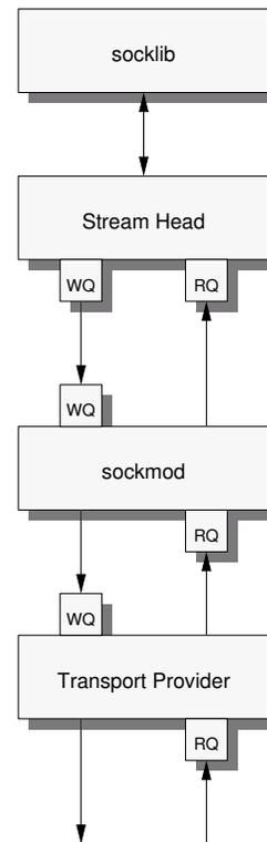
Figure 3: Socket Module
