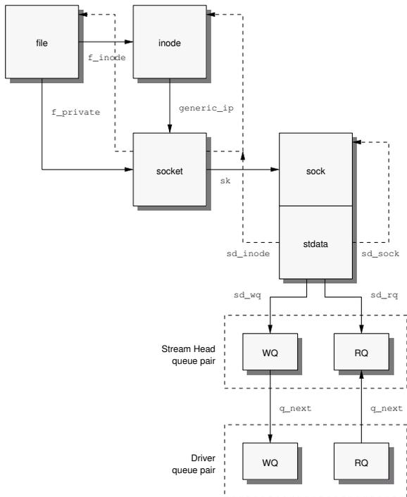
Figure 4: Socket Structures
